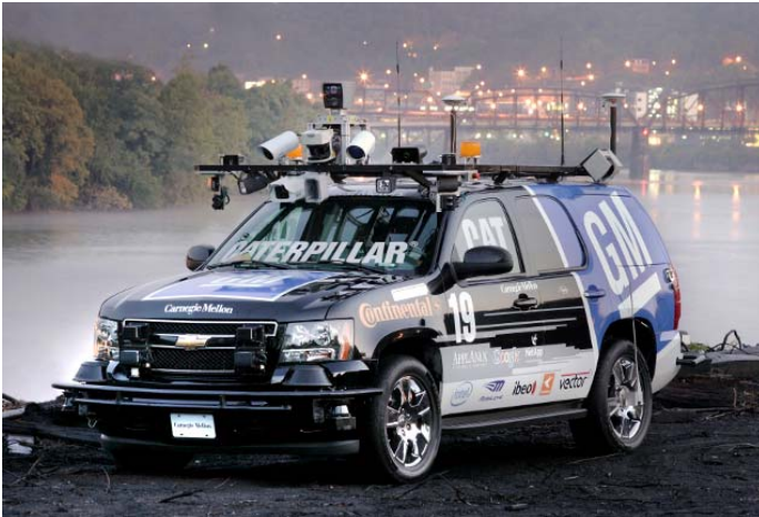
Figure 1, Boss intelligent vehicle; winner of the DARPA urban Challenge (image courtesy of Field Robotics Center, USA).
